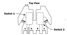
Common and B connections will close when vane is deflected, i.e., when water is flowing. Dual switches permit applications to be combined on a single detector.
