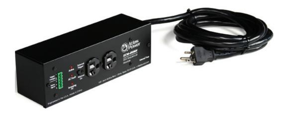
The Atlas Power ECM-20SH is a 120V 60Hz AC, 20A Single Housing (SH) Power Conditioner and AC Spike Suppressor that is designed to be used as a standalone unit or in conjunction with an Atlas Power Sequence controller, ECS-6RM or the ECS-3, up to 1000ft away.
