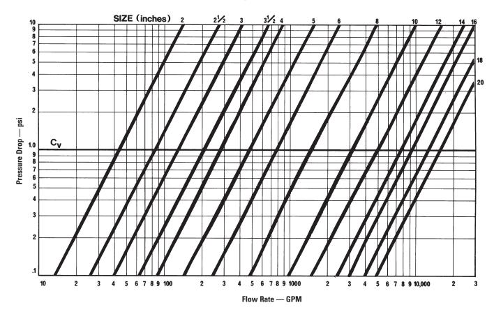
This chart is based on the flow of clean water through .033" - 1/4" inch perforated metal screens. Consult our Engineering Department for pressure drop information on steam, gases or viscous fluids.
