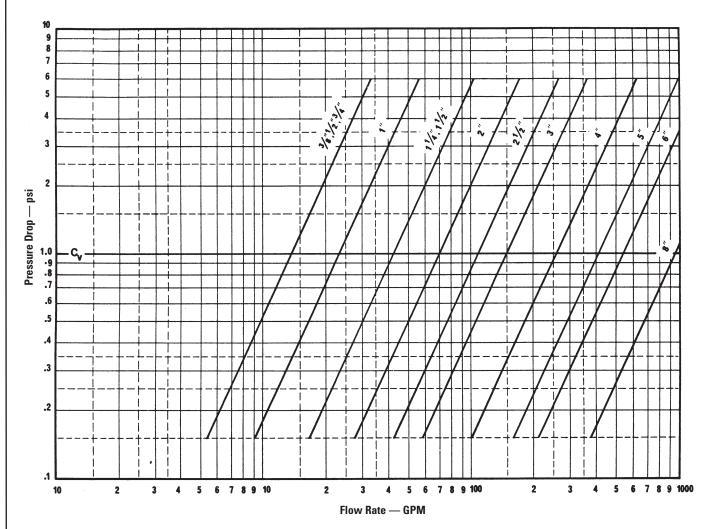
This chart is based on the flow of clean water through .033" - 1/4" inch perforated metal screens. Consult our Engineering Department for pressure drop information on steam, gases or viscous fluids.
