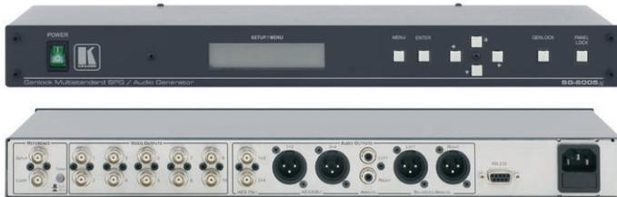
The **SG-6005xl** is a broadcast quality black burst, color bar, sync, and audio tone generator for composite video and audio applications. The unit outputs ten composite video and two AES-3id audio signals on BNC connectors, two balanced stereo and two AES/EBU audio signals on XLR connectors; and an unbalanced stereo audio signal on two RCA connectors. The unit can be genlocked to an external video source.
