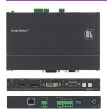
The **SID-X1** is a twisted pair transmitter and step-in commander for computer graphics video, HDMI, DVI, DisplayPort and unbalanced stereo audio signals. The unit includes a "Step-In" button that allows the local source to be routed as the active source on the main display through the main switcher.
