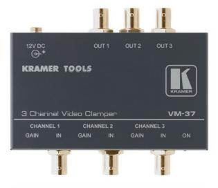
The VM-37 is a 3 channel video clamper for video, s-Video (Y/C) and YUV/RGB sources. Many video capture cards, satellite decoders and receivers, and other video and component sources ride on erroneous DC offsets that must be corrected for proper operation.
