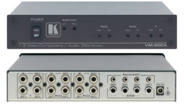
The VM-30CA is a high-performance distribution amplifier for component video (YUV), S/PDIF and unbalanced stereo audio signals. It takes one input of each signal type, provides correct buffering and isolation, and distributes the signal to three identical outputs.
