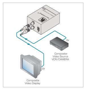
The 101L is a high-performance line amplifier for composite video signals. It provides controls to compensate for signal loss inherent in long cable runs.
