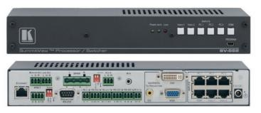
The SummitView<sup>™</sup> SV-552 processor/switcher is the heart of the system for audio and video signal distribution and room control. From one or more wall plate room controllers, the SV-552 switches up to six audio and video sources to a large screen display in their native formats, amplifies the audio to a pair of speakers, and controls room facilities such as lights and a screen.
