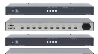
The VM-28H and VM-216H are distribution amplifiers for HDMI signals. They reclock and equalize one of 2 selectable input signals and distribute it to 8 or 16 identical outputs.
