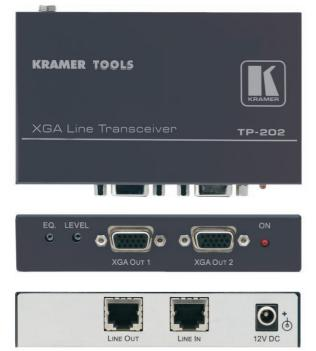
The TP-202 is a twisted pair branching receiver for computer graphics video signals with resolutions from VGA up to UXGA and higher or HDTV signals. It takes a twisted pair signal and converts it into a computer graphics video signal or HDTV signal available on two 15-pin HD outputs, and simultaneously re-transmits the original twisted pair signal to another compatible receiver.
