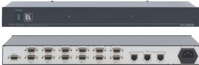
The **VP-12NHD** is a high-performance distribution amplifier for computer graphics video signals. It takes one input, provides correct buffering and isolation, and distributes the signal to 12 computer graphics outputs on 15-pin HD connectors and three twisted pair outputs.
