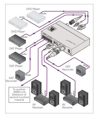
The 466N is a high-performance transcoder for digital audio signals. The unit converts one of four digital audio formats or one twisted pair input to four digital audio formats and two twisted pair outputs simultaneously.
