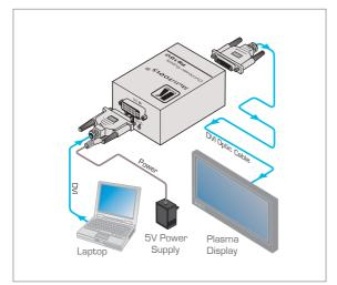
The PS-1DVI is a high-performance power supply for DVI cables. It provides 5V DC on pin 14 of the DVI plug for applications where power is not provided by the DVI source.
