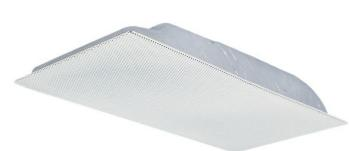
The SPK-CC838F speaker is designed for mounting in a 24-inch wide drop ceiling. The units have a perforated steel baffle and integral back box.
