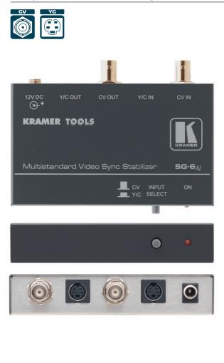
The SG-6xl is a sync stabilizer for composite video and s-Video (Y/C)signals. It identifies and corrects missing or erroneous syncs in a video signal.
