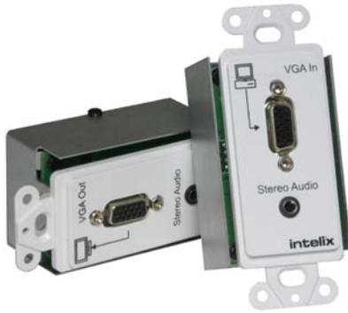
The Intelix AVO-VGA2-WP balun set transmits VGA video and stereo audio passively over two standard unshielded twisted pair cables, such as Cat 5, Cat 5e, or Cat 6. The unit eliminates costly and bulky cable while extending transmission distances.
