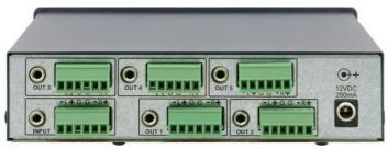
The VM-50AN is a high-performance distribution amplifier for balanced and unbalanced stereo audio signals. It takes one balanced or unbalanced stereo input and distributes the signal simultaneously to ten stereo outputs (five balanced and five unbalanced).
