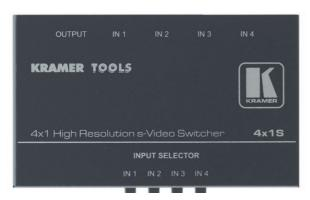
The 4x1S is a high-performance switcher for s-Video (Y/C) signals. It switches any one of four signals to a single output.
