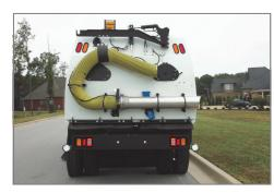
from the pavement surface, then transports it across the width of the sweeping head and lifts it into the containment hopper via a 14 inch suction tube. This highly efficient system ensures that even hard-to reach particles hidden within pavement cracks and irregularities are removed. This includes a significant amount of the
