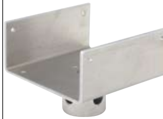
ART-CG6 6" C-grip 4.75" x 6" x 6" (12.1 x 15.2 x 15.2 cm) 1.75 lbs (0.8 kg) Adds 0.19" to length of strut
