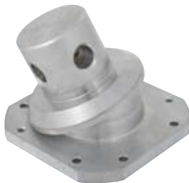
ART-S23 23° Swivel for Strut 4" x 5" x 5" (10.2 x 12.7 x 12.7 cm) 3.5 lbs (1.6 kg) Adds 2" to length of strut
