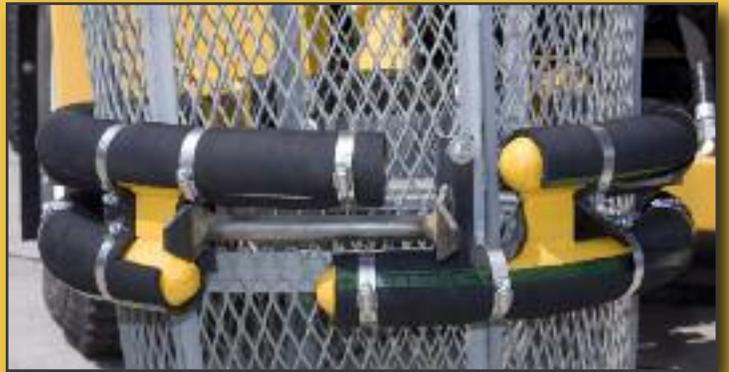
**LOADING ARM CAPACITY** Standard lift arm will grip and lift 55 to 90 gallon containers weighing up to 500 lbs. Smaller containers require optional shorter grip arms.
