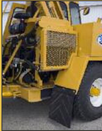
**HD MUD FLAPS** on both front wheels and with reinforced steel rims.
