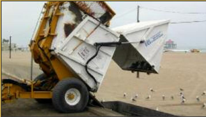
An optional self-dumping No. 7 box is available for use with stationary compactors and/or ground dumping operations.
