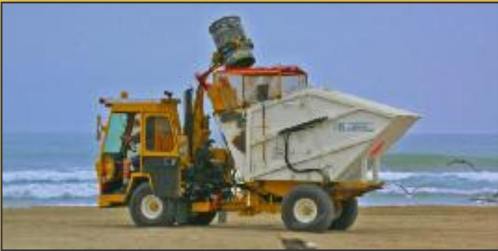
Handles most containers without damage; plastic containers, wire baskets or steel drums. Adjustable grip pressure and hydraulic lock valves maintain a secure grip.
