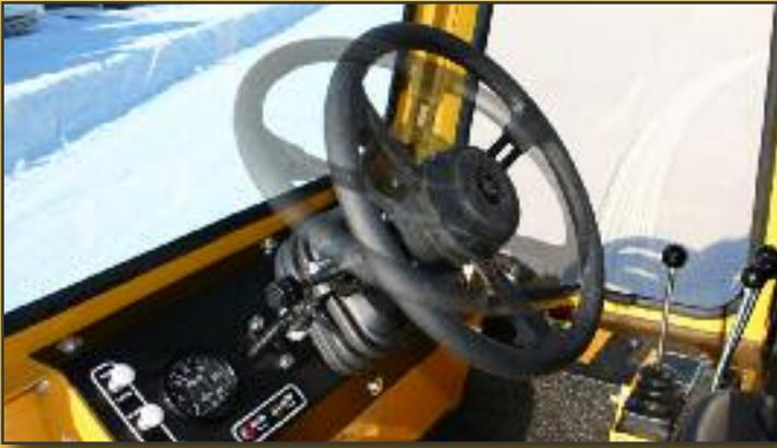
**ADJUSTABLE TILT STEERING WHEEL** with 5 positions allows for ease of driving for all Load-And-Pack users.
