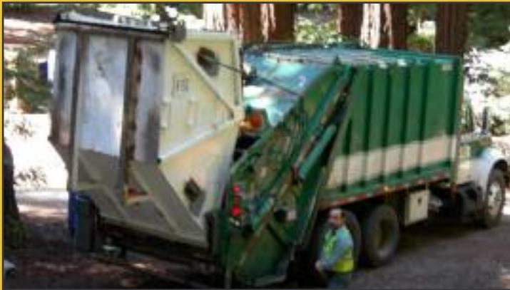
The Load-And-Pack® uses No. 7 compactor boxes with rear dumping capabilities.
