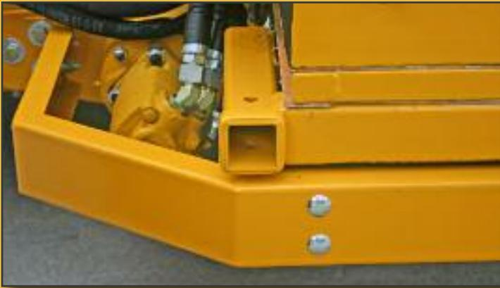
**EASY ACCESS HITCH** receiver enables using standard and towing hardware for repair or maintenance towing.
