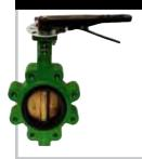
The Apollo® LC149 Contractor Grade Series Cast Iron Butterfly Valves are ideal for use in Industrial and HVAC/Mechanical applications. The LC149 Series is a lug style valve designed to be economical yet full featured. Features bronze disc and EPDM seats. Lug sizes 2″ to 12″.
