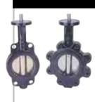
General purpose/economy ductile iron design for use in industrial and HVAC/mechanical markets. The WD141 Model is a wafer style valve; the LD141 Model is a companion lug. Both are rated at 200 psig bubble-tight shut off between flanges. LD/WD 141 Series meet MSS SP-67 and API 609 specifications. Lug sizes 2" to 24". Wafer sizes 2" to 12".
