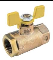
Manual shut-off valves engineered specifically for low-pressure gas service. **Canadian Standard Association** design and capacity certified with American-made quality. High-copper content body, chrome-plated ball, PTFE seats. Rated for temperatures from 32°F to 125°F at pressures of 1/2 and 5 PSIG.
