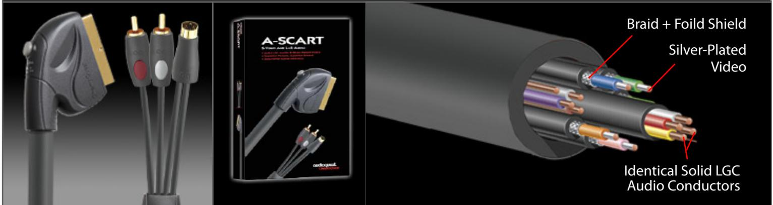
**S-VIDEO:** This two-channel (Y and C signals) high performance cable uses solid Silver-Plated Copper (SPC). Silver-Plating greatly improves high frequency performance for a fraction of the cost of solid silver. Nitrogen Injected Hard Cell Foam insulation (HCF) reduces distortion caused by the insulating material, and helps maintain a stable 75W. The combination foil and braid shield provides 100% protection.
