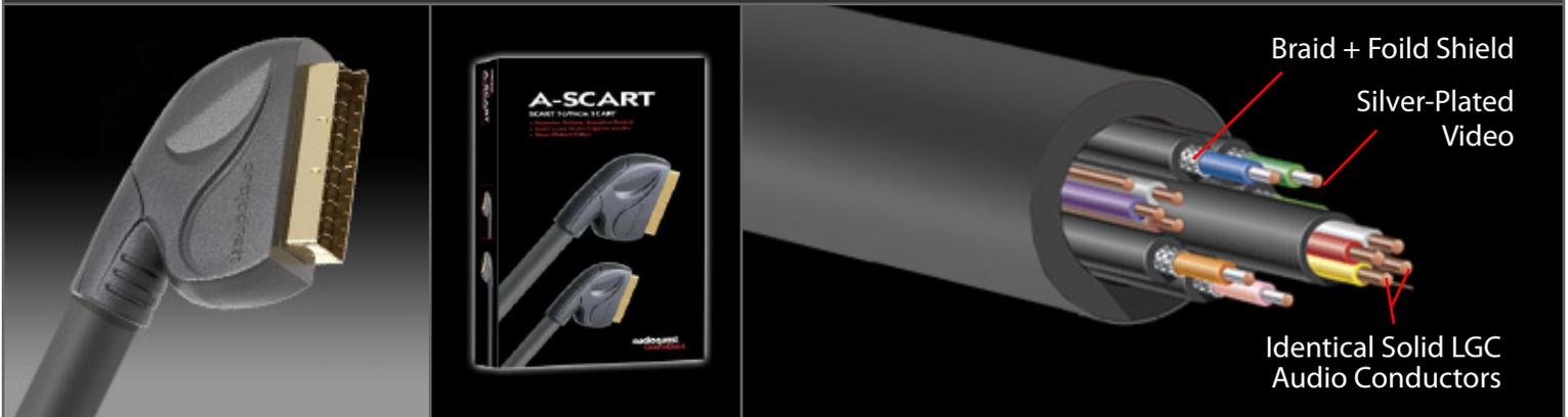
**VIDEO:** All the video conductors use solid Silver-Plated Copper (SPC). Silver-Plating greatly improves high frequency performance for a fraction of the cost of solid silver. Nitrogen Injected Hard Cell Foam insulation (HCF) reduces distortion caused by the insulating material, and helps maintain a stable 75W. The combination foil and braid shield provides 100% protection.
