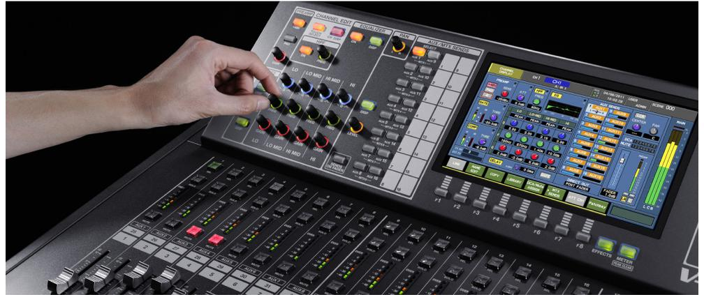
The mixing control surface shall be able to mix up to 48 channels of audio to 16 Aux buses, 8 Matrices and the LCR Main bus. The audio path from each channel shall be selectable from the pre phase, pre EQ, pre fader and post fader positions. Each channel shall have a selectable Delay setting. The mixer shall also provide 8 Matrices that accept inputs from all channels and buses. The sends to the Matrices shall be selectable from pre EQ, prefader and post fader positions.
