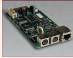
Card\* for remote shutdowns, reboots and more. Use card with optional environmental sensor\*\* to remotely monitor environmental conditions (temperature and humidity) or to control and monitor alarm/security systems. Dry contact interface works with most alarm, security and telecom devices.
