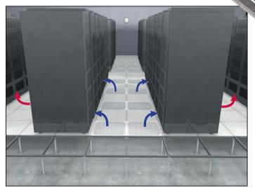
GrateAire® allows unprecedented densification of server equipment. Blue arrows indicate cool air from grate entering server, which is the cold aisle. Red arrows indicate hot air exhausted from server, forming the hot aisle.
