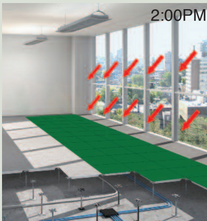
Solar load warms the panels during the day. As the panels warm the phase change material melts absorbing energy.
