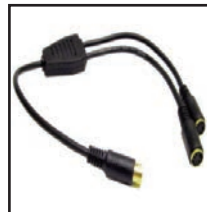
35-497A (18 in.) 35-497A-6 (6 ft.) SVHS "Y" adapter. Molded and shielded "Y" cable with 1-Male to 2-Females, pin to pin wiring. Overall length 12". For SVHS signals.
