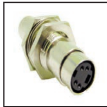
35-498 4 pin 35-498-6 6 pin 35-498-8 8 pin Bulkhead SVHS connector with 2 nut mounting. Panel mount 4 pin SVHS Female to Female. Mounts in 1/2" double "D" hole.
