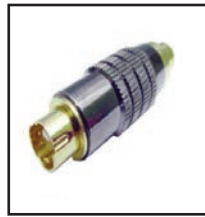
35-499 SVHS Male to RCA Female adapter. Converts SVHS signals to composite video. Bi-directional. Gold plated connectors and black chrome body.
