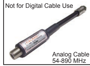
Not for Digital Cable Use Analog Cable 54-890 MHz 75-504 DC GROUND BLOCKER & ISOLATION TRANSFORMER 75 ohm In/Out, Male 'F' connector to Female 'F' connector. Eliminates hum bars or audible hum generated when A/V components are connected directly to a cable TV or satellite system. Isolates ground potential differences within an Audio/Video system without affecting the RF signal. Frequency range 54-890MHz. 6" long.
