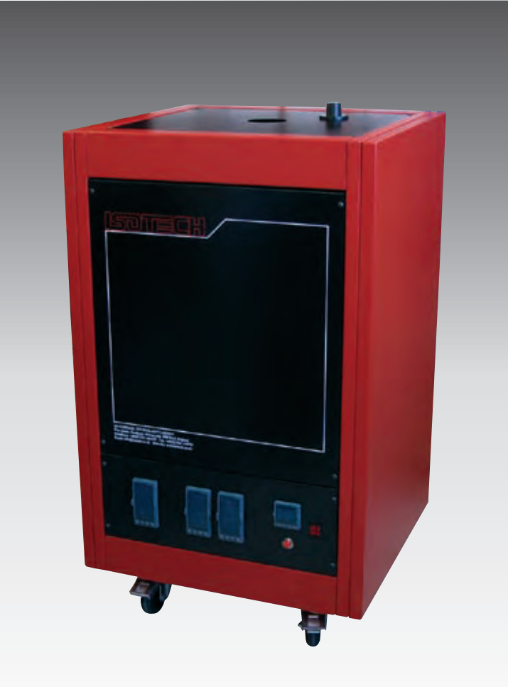
Fixed Points of: Indium 156.5985°C, Tin 231.928°C, Zinc 419.527°C, and Aluminium 660.323°C Active and Passive Safety Circuits, Equalizing Block for Comparison Calibration
