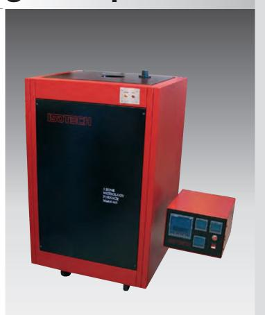
Long plateaus from Fixed Point Cells Self-Tuning controller optimizes each Fixed Points performace 3 zones controlled to compensate for end loss to give a perfect profile
