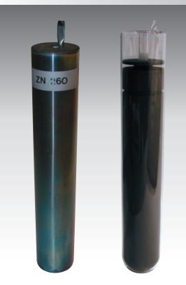
Cost effective dedicated desktop apparatus like the POTTS, "Points on the Temperature Scale" can be used to automatically bring the cell to the plateau. These simple to use systems conveniently provide long flat plateau for low uncertainty calibration of thermometers.
