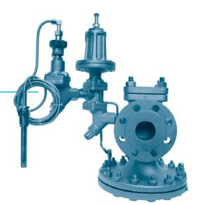
Low Pressure Temperature Pilot must be used in conjunction with a low pressure main valve for applications where inlet steam pressure is <u>less than 15 PSIG.</u>
