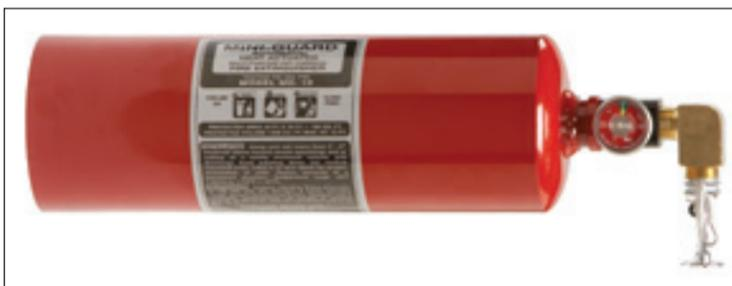
The Mini-Guard automatic spot protection extinguishers are designed, constructed, and tested to the same engineering standards as our portable fire extinguishers. Available in horizontal or vertical configurations, the units can be charged with multipurpose (ABC) dry chemical or Halotron agents and are fitted with a detection sprinkler head that is rated at 165° F.
