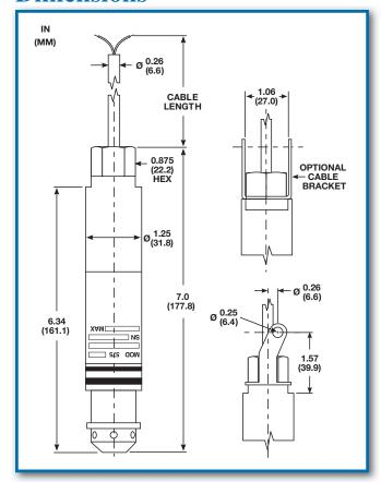
Housing Type: 316 stainless steel Nut/Washer Type: 316 stainless steel Cable Grommet: Viton standard. Please contact factory for other options.
