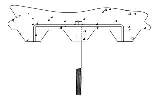
Before pouring concrete, locate the Figure 284 on deck so legs rest in "valleys" of form. Drill hole in deck for bolt.
