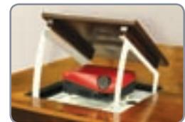
The Phantom is supplied with a universal-style bracket that allows for easy attachment of a variety of projector models. Two Phantom models to choose from that fit most projectors up to 26 lbs. The Phantom motor is a 24V DC low voltage motor, which allows for easier control and wiring of the lift.
