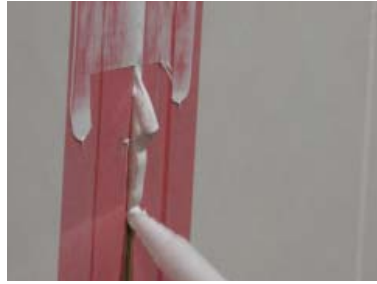
Figure 19: Bump adhesive in to previous section
