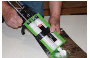
Figure 13: Leveling the Plungers
