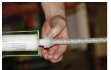
Figure 14: Attach Static Mixing Tip
