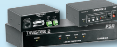
TWISTER 2 Systems for Transmission of Data, IR, Audio and Video Signals over Twisted Pair
