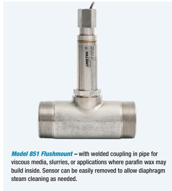
**Model 851 Flushmount** – with welded coupling in pipe for viscous media, slurries, or applications where paraffin wax may build inside. Sensor can be easily removed to allow diaphragm steam cleaning as needed.
