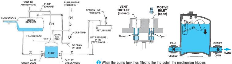
When the pump tank has filled to the trip point, the mechanism triggers, opening the motive gas inlet valve and simultaneously closing the vent valve. This allows motive pressure to enter the pump body, which drives the condensate thru the outlet check valve into the condensate return line. During the discharge cycle, the liquid level and the float inside the pump tank drop.
