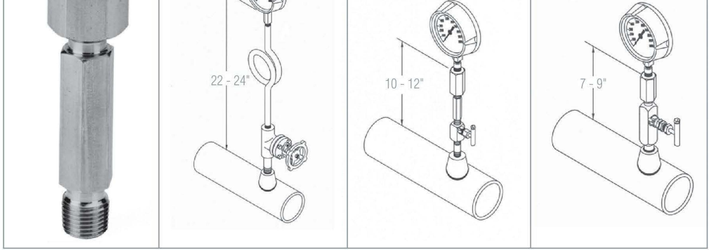
Hex gauge syphons act as thermal and liquid seal barriers between hot process vapors (such as steam and heat transfer fluids) and the gauge pressure instrument. It is designed to replace the large installation space requirements of the traditional "pigtail" syphon, providing maximum instrument protection in half the space. This reduced radius minimizes weight and deflection stress at the primary valve.
