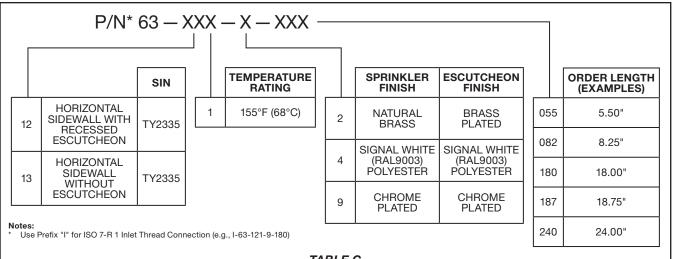
TABLE C RAPID RESPONSE SERIES LFII DRY-TYPE RESIDENTIAL HORIZONTAL SIDEWALL SPRINKLERS PART NUMBER SELECTION
