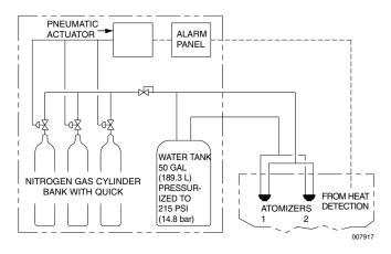
The above figure provides a system schematic. The engineered AQUASONIC System provides a less complex alternative to high pressure water mist systems. It is primarily comprised of a pre-packaged AQUASONIC Supply Skid containing both compressed nitrogen and stored water which upon actuation automatically supplies the necessary quantity of each to the AQUASONIC Atomizers.
