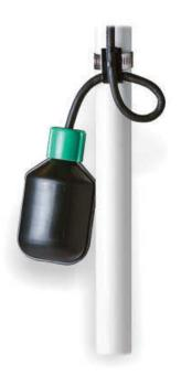
This control switch is used to accurately monitor high (normally open) or low (normally closed) liquid levels to activate pump control panels and alarms in water and sewage applications. It features a green colored cap for easy identification of SPDT control switch. This switch can be wired to work in either normally open or normally closed applications.
