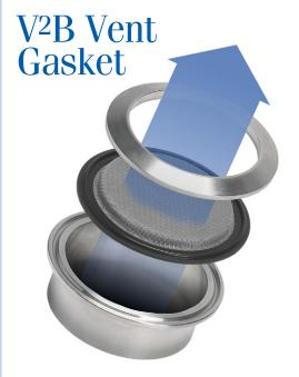
The Rubber Fab V<sup>2</sup>B Vent Gasket provides vacuum and pressure relief for **pharmaceutical** and **food/beverage processing** tank venting when **airborne particulate removal is required**. A 200 mesh screen combined with a 14 mesh screen of **sintered construction** creates a cost effective alternative to expensive vacuum breakers and venting systems.
