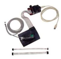
These kits enable upgrading firmware in KMDigital and BACnet controllers, the BAC-5050 router, and the KMD-5540 series CommTalk protocol interfaces. The kits include the relevant programming pod and cables. Both kits also have adapter plates for the three types of FlexStat backplates as well as adapter CO $_2$  gas tubing for calibrating BAC-14xxxx models. The HTO-1104 is for all models, and the HTO-1103 is for FlexStat models only.
