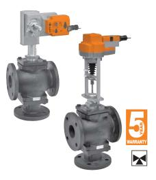
**Mode of Operation** The control valve is operated by an electronic actuator that responds to a standard voltage for on/off control, a proportional VDC/4...20 mA, or 3-point control system. The actuator will then move the plug of the valve to the position dictated by the control signal thus changing the flow.
